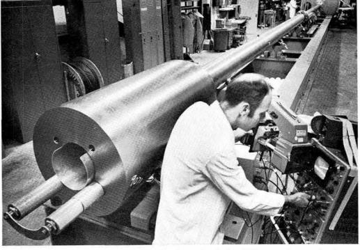
BIG GUN — Bob May, foreground, and Bob Hardy (both 5163), near impact chamber, adjust instrumentation for Sandia's new high-velocity gun facility. The gun is 87 feet long with a 3.5-inch bore. It can fire a two-pound projectile and achieve impact velocities of 8000 fps in materials research programs.
